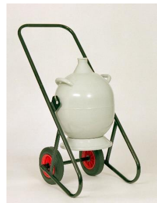
Figure 8: Dewar mounted on a trolley
