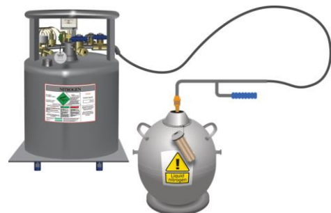
Figure 9: Decanting liquid nitrogen
