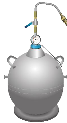
Figure 8: An example of a liquid withdrawal device. Additional security provided with a restraining wire.
