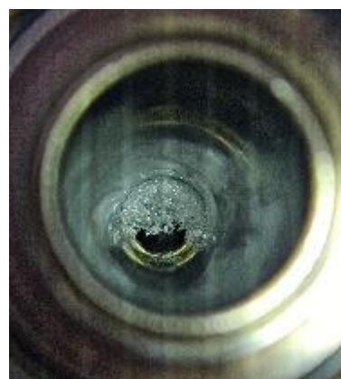
Figure 12: An example of an ice plug forming
