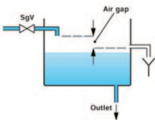
**Type AF air gap with circular overflow.** This provides back-flow protection to fluid category 4. The dimension of the air gap between the discharge point and the 'critical water level' (water level two seconds after closing the inlet) must meet the minimum requirements for the standard.
