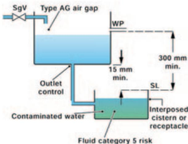
**Type AUK1 air gap with interposed cistern.** This provides back-flow protection to fluid category five. The air gap in the cistern must meet the requirements for a type AG air gap (British Standard BS6281: Part 2).
