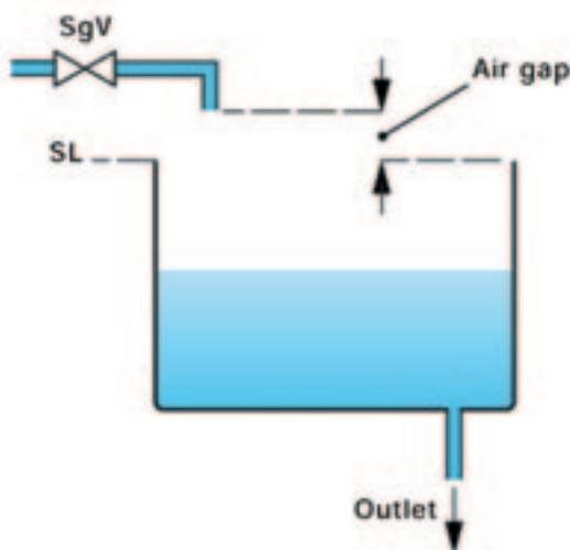
**Type AA air gap, with unrestricted discharge.** This provides back-flow protection to fluid category five. The discharge point is located above the spillover level (SL) of the receptacle. The minimum distance between the discharge and the spillover level must meet the requirement for a type AA air gap.
