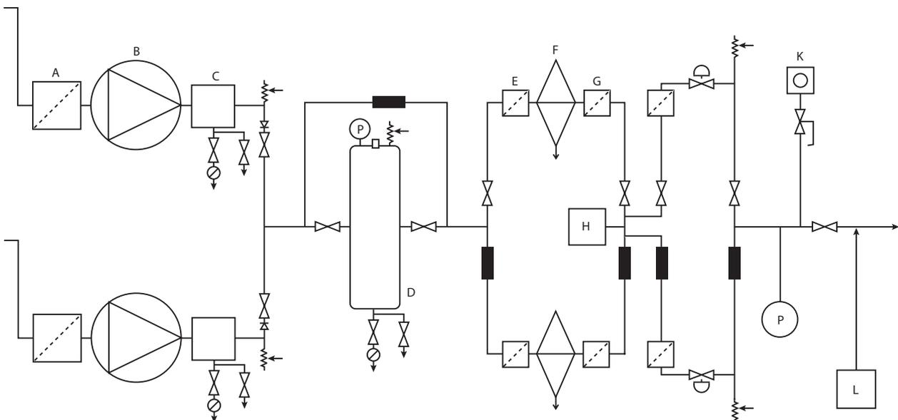
Figure 3.3 A small simplex air plant with single column regenerative dryer
