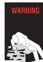
For any enclosed load space, a warning label shall be displayed at all access points where it can easily be seen, highlighting the danger of asphyxiation (the letters on which shall be a minimum of 25 mm high).
