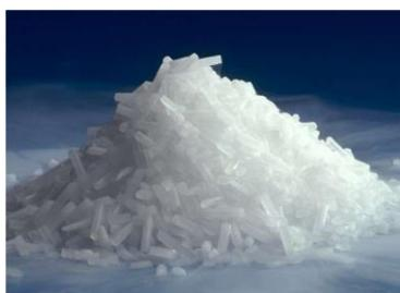
In its solid form it is often used as a refrigerant or coolant when transporting and storing other temperature critical products. Solid CO<sub>2</sub> is manufactured in the shape of pellets, slices or blocks and may be supplied loose or in insulated containers.
