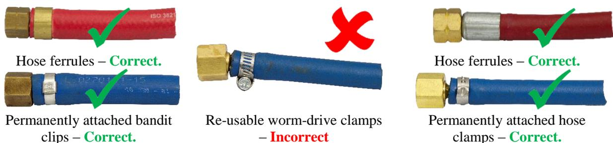
**Figure 6:** Hose connections
