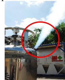
Gas venting from a vacuum protection device.
