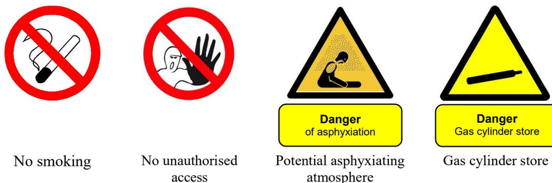
**Figure 1:** Examples of safety signs and warning notices
