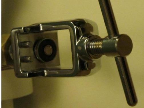
**Figure 1:** Pin index yoke
